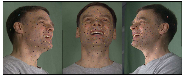
Figure 1. Colored beads have been glued on the subject's face along Langer's lines so as to cue geometric deformations caused by main articulatory movements when speaking.
