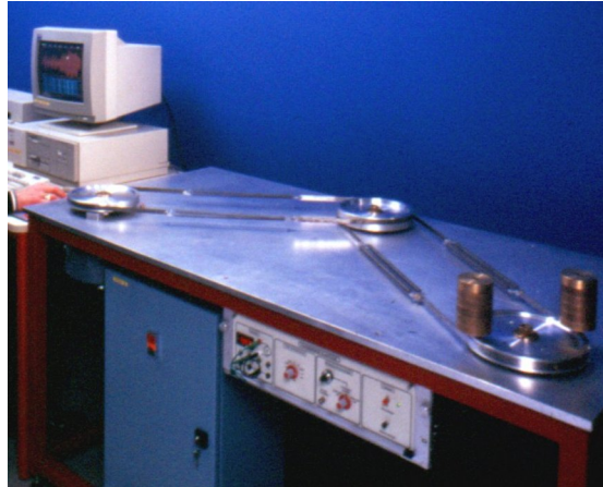
Figure 1b. View of the flexible transmission system
