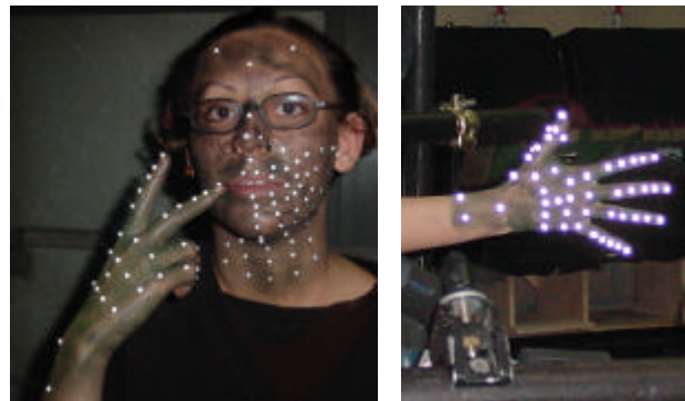
Figure 3. Our female FMCS user and the reflective markers used for the dynamic corpus. She wears 50 markers on her right hand and 63 markers on her face, mainly on her left side.
