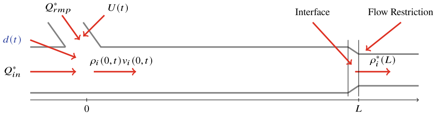
Fig. 1 Heterogeneous vehicle traffic on a road with disturbances at the inlet boundary and a velocity drop in the right boundary
