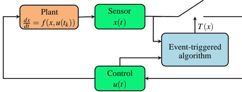
FIG. 1. Control scheme with an event-triggered algorithm.
